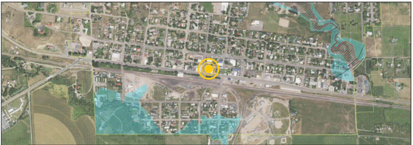
FEMA Floodplain Map: Project site is in Flood Zone "X" (minimal hazard)
